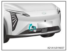
Insert the towing hook into the towing port, turn it clockwise and tighten it.
