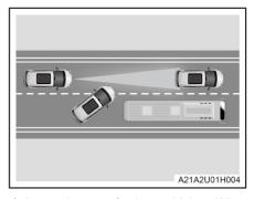
♦ Lane change of other vehicles. When a vehicle in the adjacent lane goes into the ego lane, if it does not enter the detection range, it could not be detected by the RPA sensor, thus resulting in a response lag of ACC.
