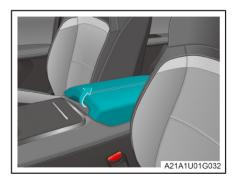
Pull up the central armrest as arrowed, and open the central armrest box.
