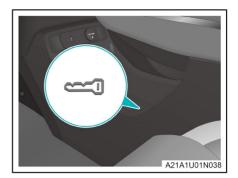
When the battery of smart key runs out or is low, enter the vehicle, place the smart key at the mark, depress the brake pedal and power on the vehicle, and then move the gearshift lever as soon as possible start the vehicle.
