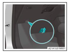
Pull up the hood release lever in the cab, and then the hood 'clicks' and pops up slightly.
