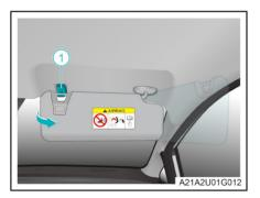
After the sun visor is turned down, disengage the fastening hook 1 and turn the sun visor to the side window to block the dazzling light from the side.
