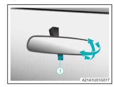
Adjust the interior rearview mirror up and down, left and right to the best rear view position.
