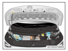
Open the hood, and check the coolant level in the expansion tank in the area marked with frame as shown. If it is below the "MIN" mark, please fill the expansion tank with coolant to the level between the "MIN" and "MAX" marks in time.
