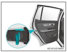
Insert the mechanical key into the keyhole in the door lock, turn the key clockwise to the locked position, pull out the mechanical key, and close the door to lock the door.
