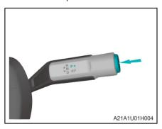
After the vehicle comes to a full stop, press the "P" button to shift to "P" position. Then the EPB is automatically enabled.
