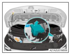
The motor compartment fuse box is located at the right rear of the motor compartment (facing the front end of the vehicle). You can open the hood, and press the buckles on both sides of the fuse box while pulling up the fuse box cover to check the motor compartment fuse.
