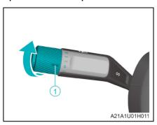
Turn the wiper control knob up or down from the O position, so that the front wiper position icons are aligned with the wiper control knob position reference icons ① in turn, and the front wiper mode can be selected. The specific control is as follows:
