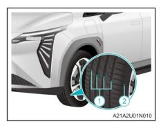
There is a raised "tread wear indicator" ① on the front of the tire. If the tread pattern wears to the indicator surface, the tire can no longer be used safely and must be replaced immediately.
