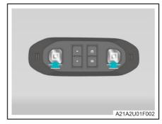
Press a front reading lamp to turn on/off the front reading lamp of concerning side.
