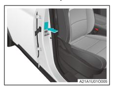
The manufacturer's nameplate is pasted near the front door lock catch of B-pillar on the front passenger side.
