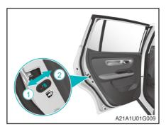
When a child takes a rear seat, please move the switch to locking position ① before closing the door. At this time, the door cannot be opened from inside, so as to prevent the child from opening the door unexpectedly.
