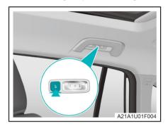
When you press the rear reading lamp switch on both sides, the rear reading lamp of concerning side will be turned on/off.
