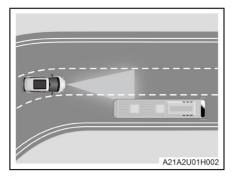
Driving out of a curve. During driving out of a long curve, as ACC will calculate the lane in advance, the radar may respond to the vehicles in adjacent lanes and apply the brake of your vehicle. This braking process can be interrupted by depressing the accelerator pedal.
