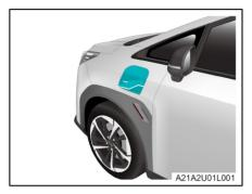
Unlock the vehicle, press the rear edge of the charging inlet cap located on the left side of the vehicle to open it.
