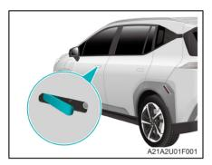
Unlock the vehicle, and after the flush-fit door handle extends automatically, pull the handle to open the door.
