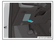
The instrument panel fuse becomes accessible after the driver side lower quard plate assembly is removed.
