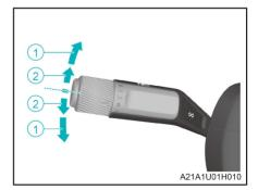
Turn signal: Move the light/wiper control lever to ① position to make the corresponding side turn signal lamp flash continuously.
