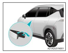
Insert the mechanical key into the keyhole, and turn the mechanical key to unlock or lock the door.
