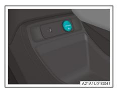
Enter the vehicle, lift the 12V power outlet cover and connect an electrical consumer at the same time to use the 12V power supply.
