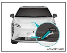
Stand in front of the vehicle (facing the front end of the vehicle), put your hand into the area to turn the secondary release lever as arrowed in the figure, and then lift the hood upward at the same time
