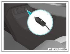
4. Insert the power plug of the inflator pump into the power outlet.
