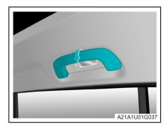
When the vehicle is running fast or on a bumpy road, the safety handrails can be used to keep the body balanced.
