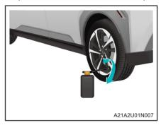
2. Shake the tire sealer, and screw the tire sealer connector into the tire valve.
