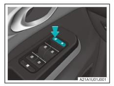
The locked door can be unlocked by pressing the unlocking end of the central locking switch inside the vehicle.
