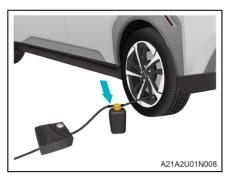
Connect the connector of the inflator pump to the bottle opening of tire sealer.
