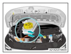
Open the hood, and check the brake fluid level in the brake fluid reservoir. If it is below the "MIN" mark, please fill the brake fluid reservoir with brake fluid to the level between the "MIN" and "MAX" marks in time
