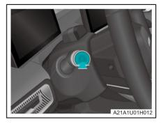
Press the front wiper washer button to have the front washer nozzle spray washer fluid. After the wiper control lever is released, the front washer nozzle stops spraying the washer fluid, the wiper operates several times, and then operates once after a period of time and stops.
