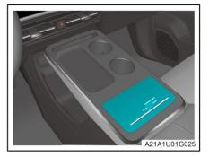
Press the area indicated by the arrow on the console storage box to open it.
