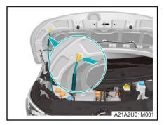
Take out the stay bar and insert it into the position as shown in the figure to fix the hood.
