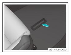
♦ The VIN is engraved at the floor in front of the front passenger's seat.
