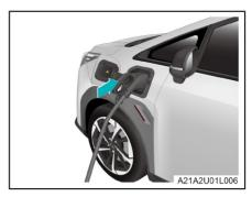
Insert the charger as arrowed. After the charger is successfully connected, all turn signal lamps are on for a long time and then go off, and the charger indicator lamp for on the instrument cluster comes on.
