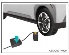
Start the vehicle, and turn on the power switch of the inflator pump to start tire repair.
