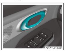
The locked door can be unlocked by pulling the door inside handle.
