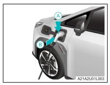
3. While pressing the unlocking button of the charger in the direction of arrow A, insert the charger in the direction of arrow B. After the charger is successfully connected, all turn signal lamps are on for a long time and then go off, and the charger indicator lamp on the instrument cluster comes on.
