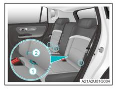
There are four ISOFIX anchorages ① provided between the rear seat back and the rear seat cushion for installation of child seat. Label ② is used to indicate the position of ISOFIX anchorage.
