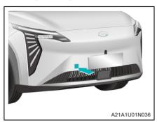
1. Open the towing cover at the lower right of the front bumper.
