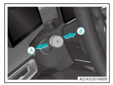
After the headlamp is on, push the light/ wiper control lever in the direction of arrow A to switch the headlamp to the high beam, and pull back the light/wiper control lever in the direction of arrow B to turn off the high beam
