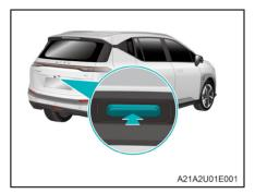
When you press the liftgate micro switch with smart key in hand or after the vehicle is unlocked, the liftgate will be unlocked.
