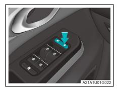
When doors are closed, press the locking end of the central locking switch inside the vehicle to lock all the doors.
