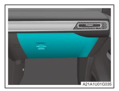
Press the glove box switch to open the glove box.
