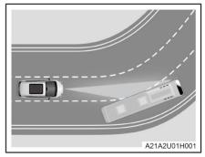
Driving through a curve. During driving through a curve, the RPA sensor may fail to capture the vehicle ahead, or may respond to vehicles in adjacent lanes. In this case, the ACC may brake the vehicle, reduce the vehicle speed, or make no response to the vehicle ahead. At that time, step on the brake pedal or manually cancel ACC.
