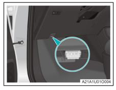
The OBD DLC is located at the lower left rear of the instrument panel. Data such as the vehicle identification number (VIN) and vehicle status information can be read by connecting a special diagnostic scan tool to the OBD DLC.
