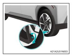
1. Park the vehicle in a flat and safe place, and remove the tire valve cap.
