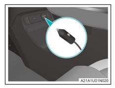
3. Insert the power plug into the power outlet.
