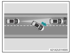
♦ If the target vehicle in front is driven out suddenly and a stationary vehicle appears at close range, the radar sensor and brake actuator will incur a response lag, causing delayed braking response.
